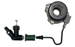
Figure 2: Hydraulic line, guide, and connection parts from the vehicle manufacturer
